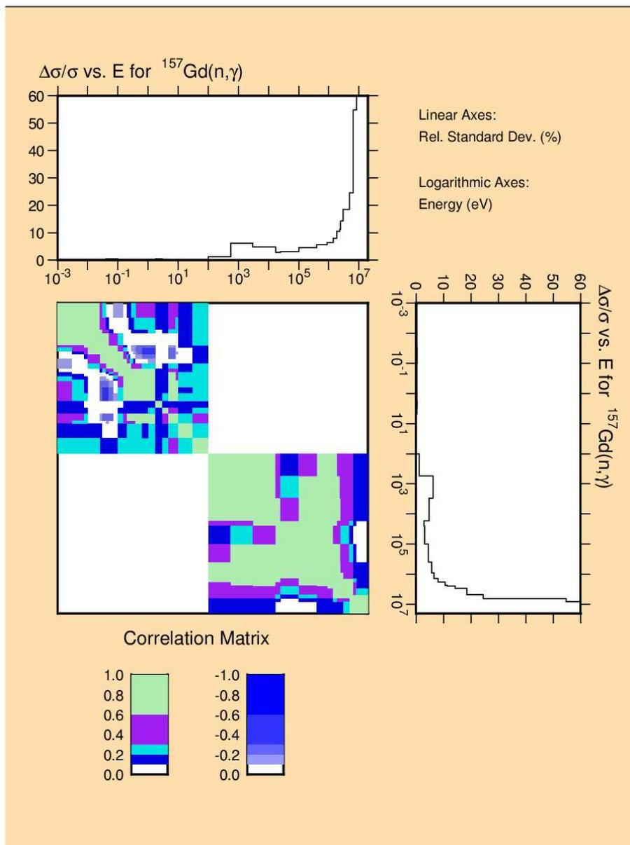
reaction models can only be used above the resonance region. The division is naturally propagated also on the covariance data. Resolved resonance, unresolved resonance, and fast neutron regions are always assumed to be uncorrelated that results in correlations matrices partitioned into three isolated squares along the diagonal.
