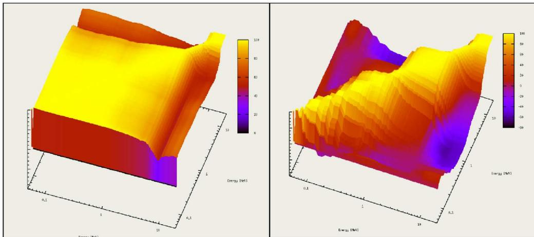
This expectation is confirmed by KALMAN/EMPIRE calculations that naturally include both model-based prior and experimental data. In Fig. 3 we compare self-correlations for neutron capture cross sections on  $^{157}\text{Gd}$  obtained under two scenarios: (i) pure model calculations and (ii) model calculations together with experimental data for neutron capture. One observes that
