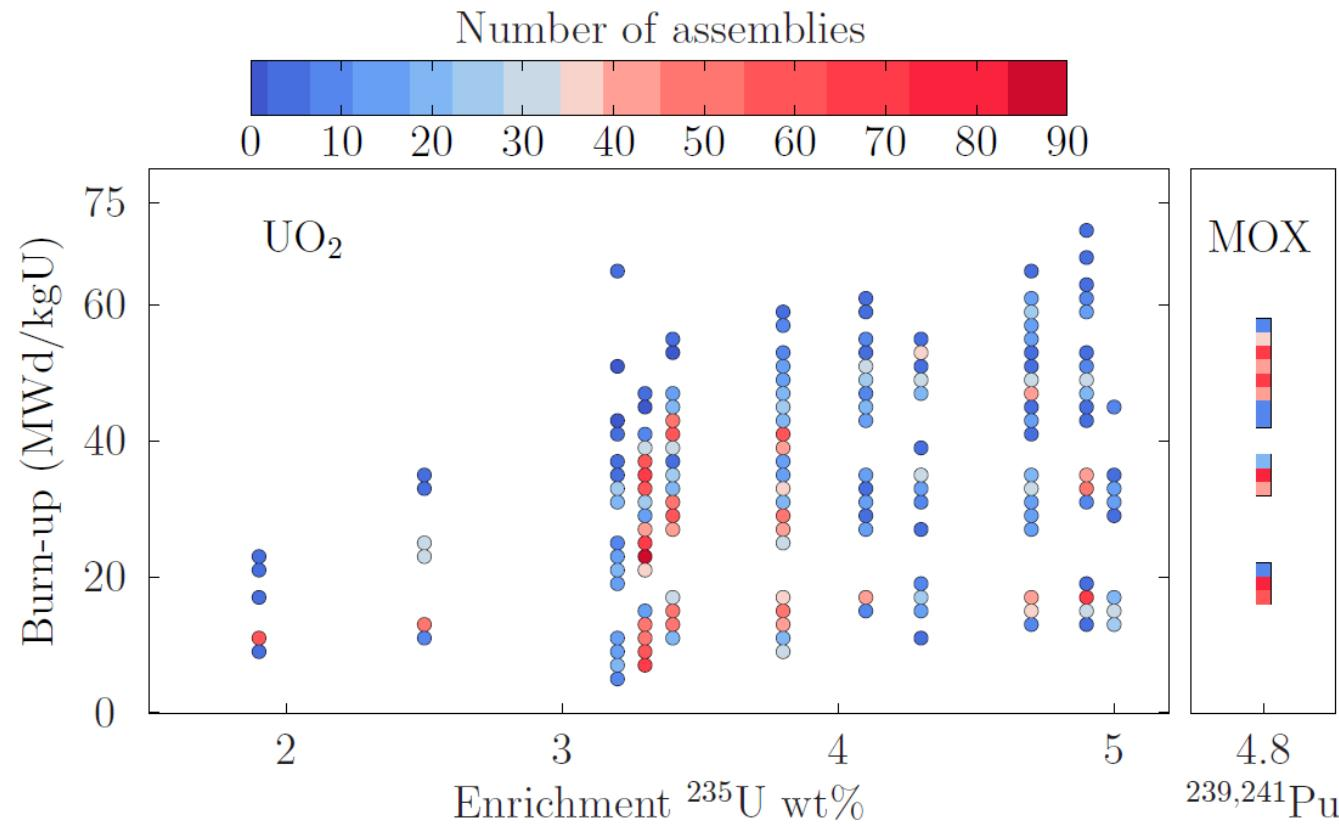
Fig. 1. Total number of fuel assemblies considered in this work from a specific Swiss PWR power plant, over 34 cycles (5378 UO<sub>2</sub> and 640 MOX assemblies). All assemblies are considered at the end of each cycle, being discharged or not.
