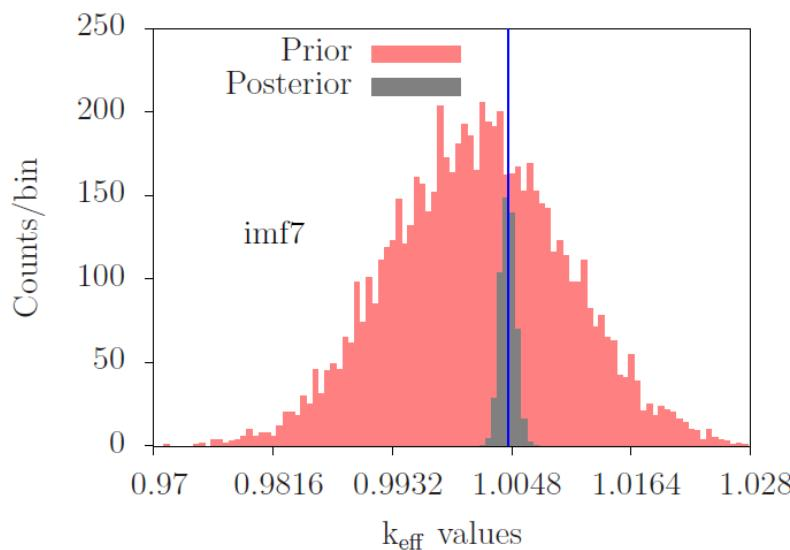
**Fig. 12.** Prior and posterior distributions of  $k_{\text{eff}}$  for imf7 benchmark. The blue line indicates the experimental value.
