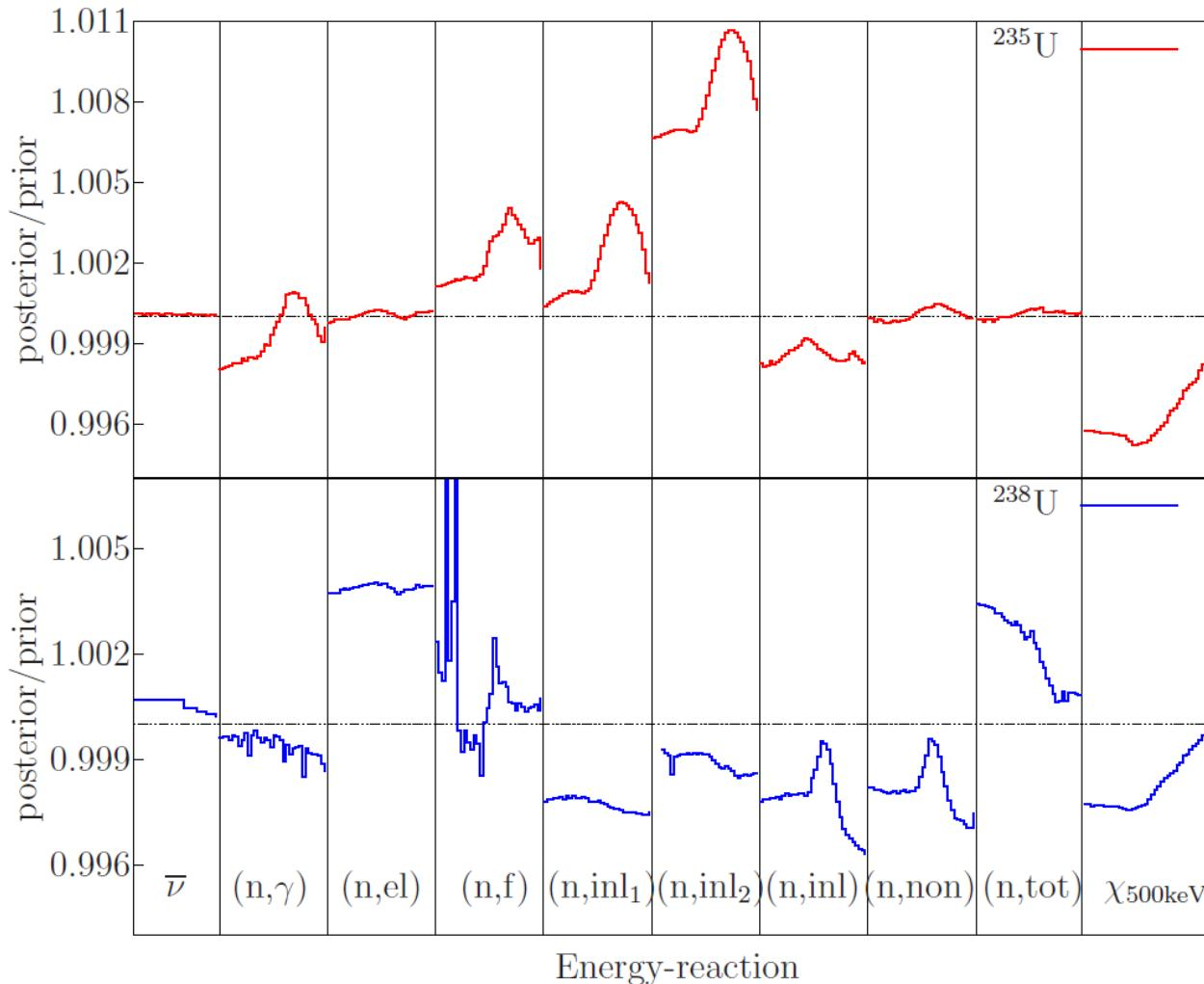
**Fig. 9.** Ratio of cross sections (and  $\bar{\nu}$  and  $\chi$ ) for the post-adjusted (*a posteriori*) over the prior. The cross sections,  $\bar{\nu}$  and  $\chi$  are presented from 100 keV to 6 MeV on a logarithmic scale.
