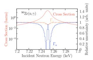
**Fig. 1.** Relative cross section uncertainties from  $\Gamma_{\gamma}$  and  $\Gamma_n$  (right scale) and cross section (left scale) for  ${}^{90}$ Zr(n, $\gamma$ ) for the single 7.251 keV resonance.
