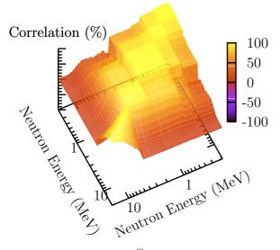
**Fig. 4.** Correlation matrix for the <sup>90</sup>Zr neutron capture cross sections in the fast neutron region obtained with the EMPIRE-KALMAN method without experimental data.
