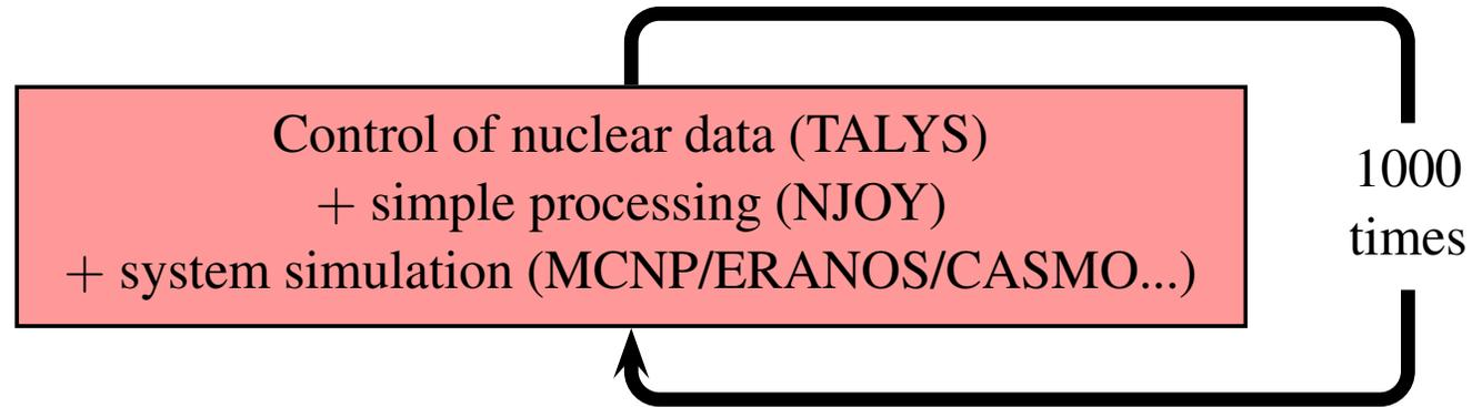
For each random ENDF file, the benchmark calculation is performed with MCNP. At the end of the  $n$  calculations,  $n$  different  $k_{\text{eff}}$  values are obtained. In the obtained probability distribution of  $k_{\text{eff}}$ , the standard deviation  $\sigma_{\text{total}}$  reflects two different effects:  $\sigma_{\text{total}}^2 = \sigma_{\text{statistics}}^2 + \sigma_{\text{nuclear data}}^2$ .
