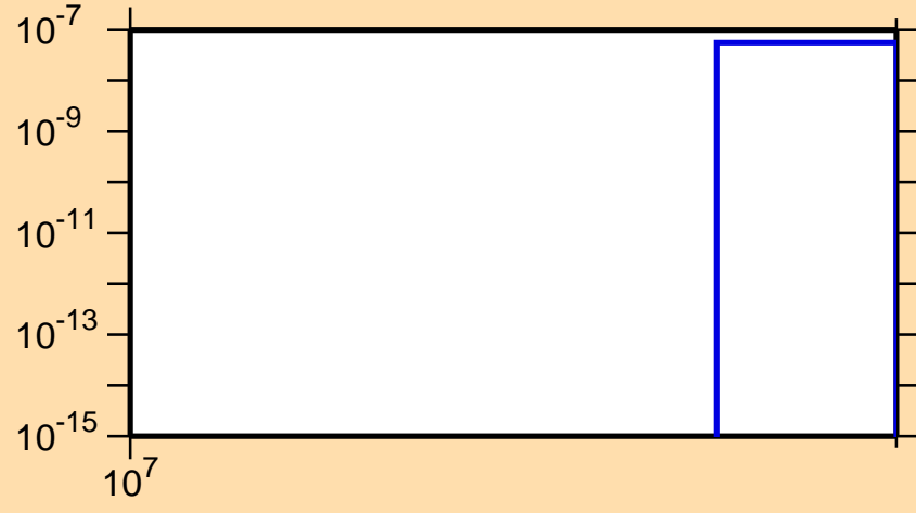
\sigma vs. E for ^{201}\text{At}(n,3n\alpha)
