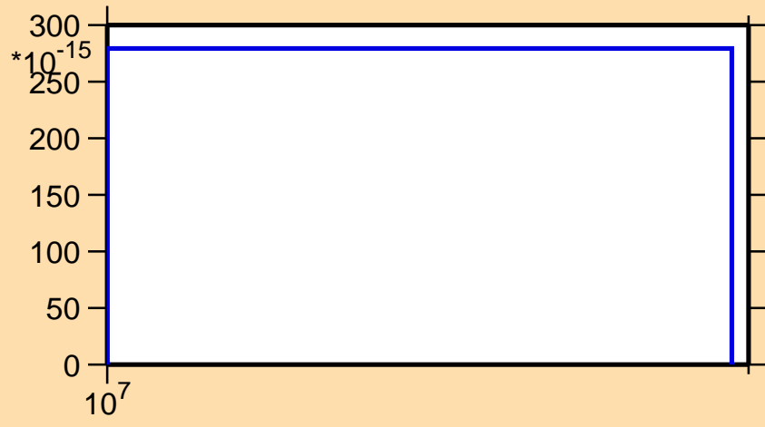
\sigma vs. E for ^{128}\text{Sb}(n,2n\alpha)
