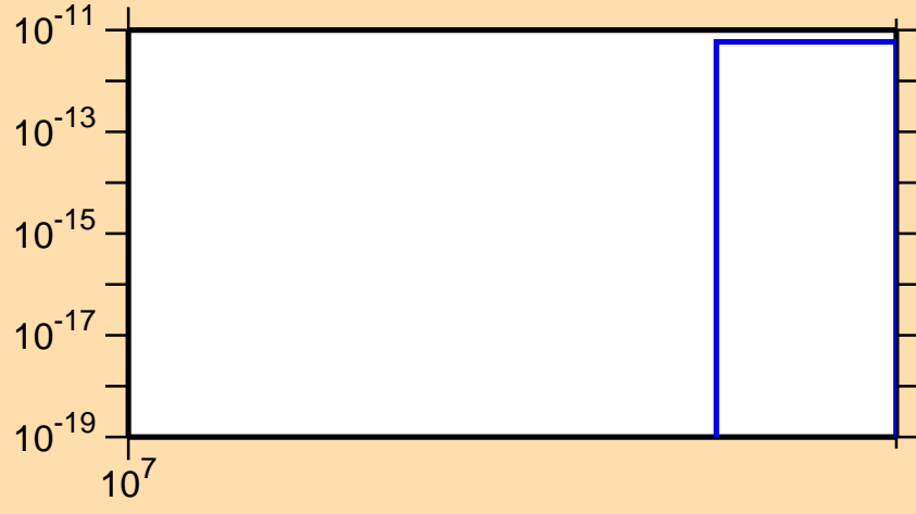
\sigma vs. E for ^{153}\text{Sm}(n,3n\alpha)
