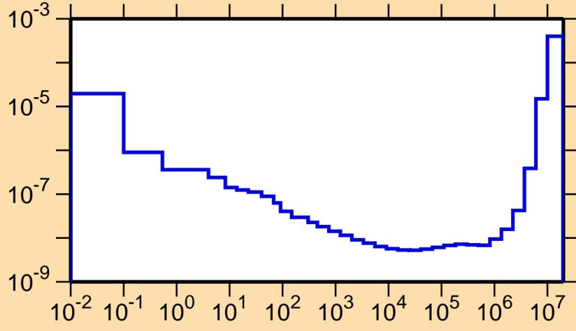
$\Delta\sigma/\sigma$  vs. E for  $^{236}\text{Am}(n,p\alpha)$
