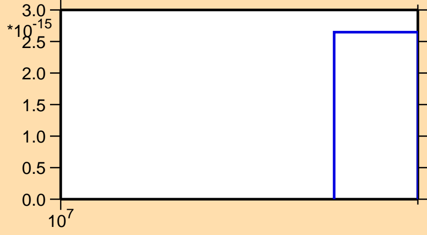
\sigma vs. E for ^{122}\text{Cd}(n,\text{nd})
