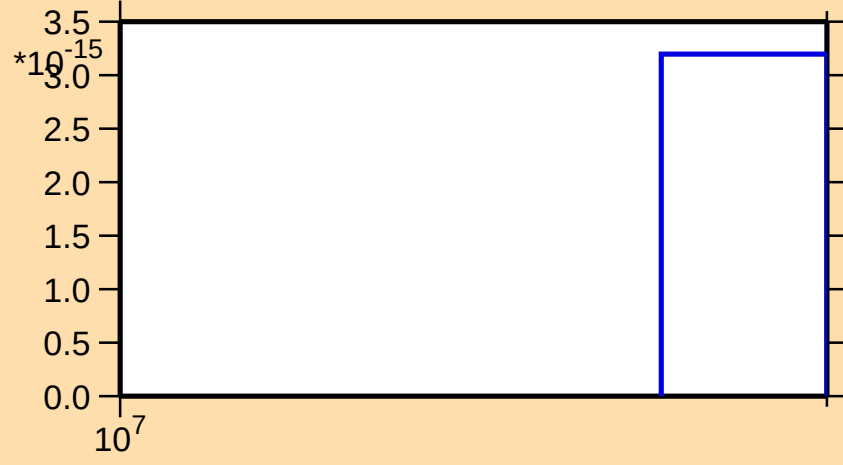
\sigma vs. E for ^{60}\text{Fe}(n,\text{nt})
