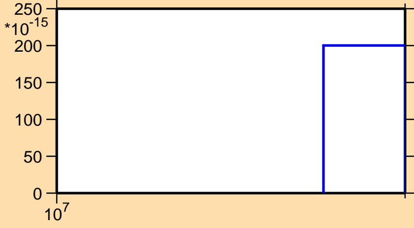
\sigma vs. E for ^{87}\text{Nb}(n,nt)
