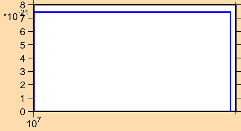
\sigma vs. E for ^{209}\text{Pb} (mt 42)
