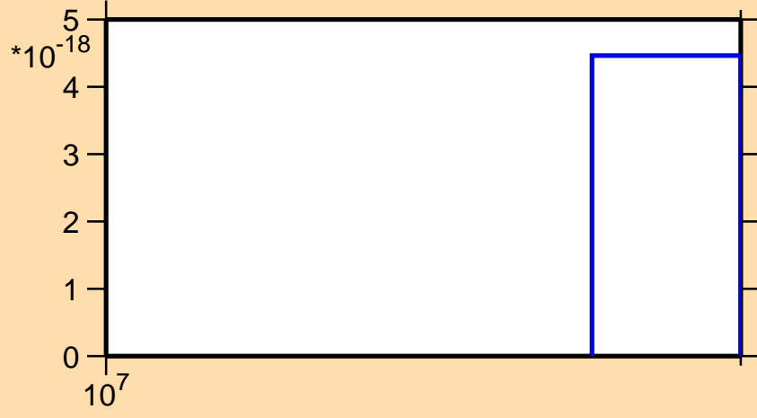
\sigma vs. E for ^{228}\text{Ra} (mt 42)
