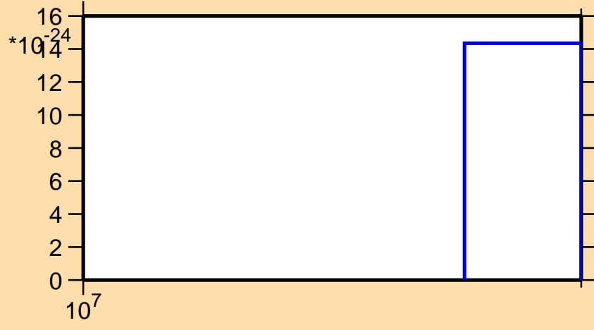
\sigma vs. E for ^{126}\text{Sb} (mt 11)
