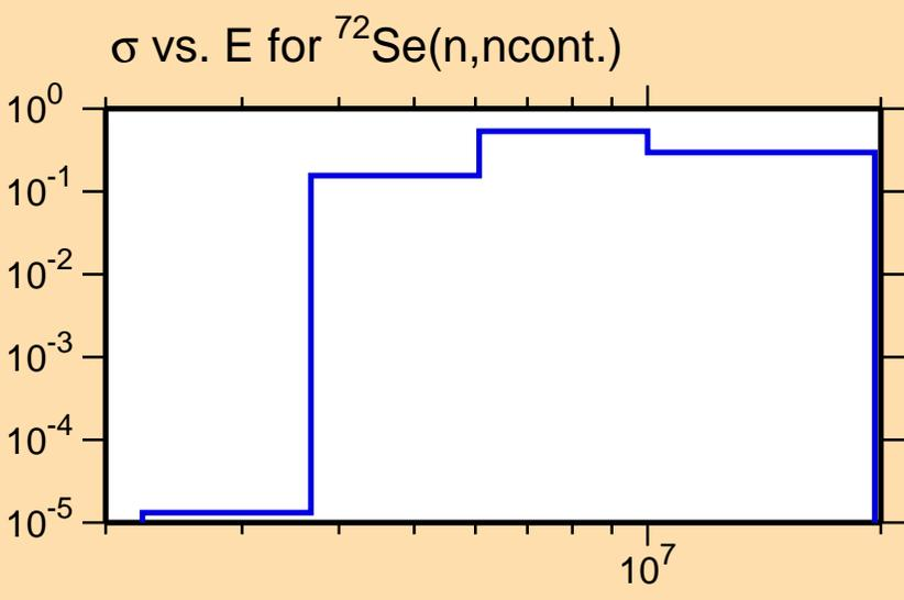
$\sigma$  vs.  $E$  for  $^{72}\text{Se}(n,n\text{cont.})$
