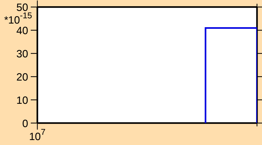
\sigma vs. E for ^{125}\text{Sn}(n,\text{nt})
