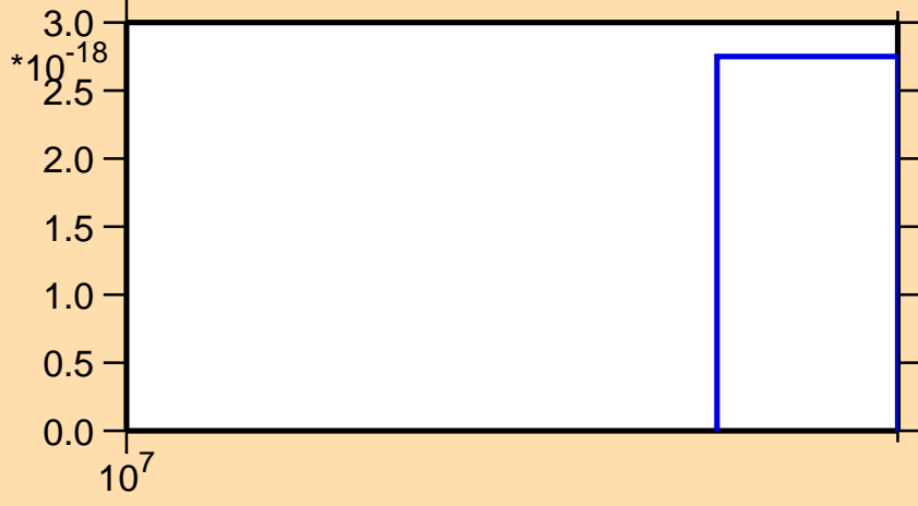
\sigma vs. E for ^{205}\text{Hg} (mt 11)
