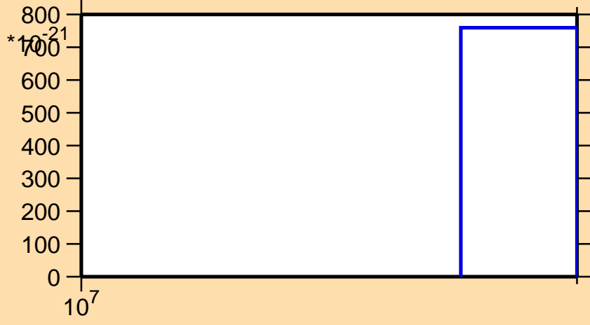
\sigma vs. E for ^{68}\text{Ni}(n,2n\alpha)
