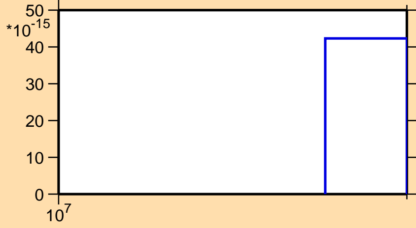
\sigma vs. E for ^{118}\text{Pd}(n,\text{nd})
