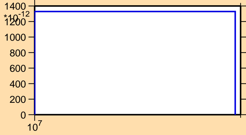
\sigma vs. E for ^{48}\text{Ti}(n,\text{He}3)
