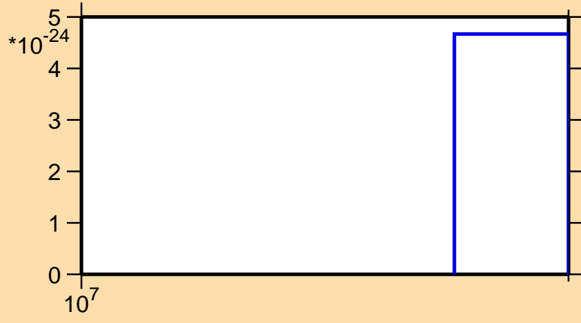
\sigma vs. E for ^{180}\text{Hf} (mt 42)
