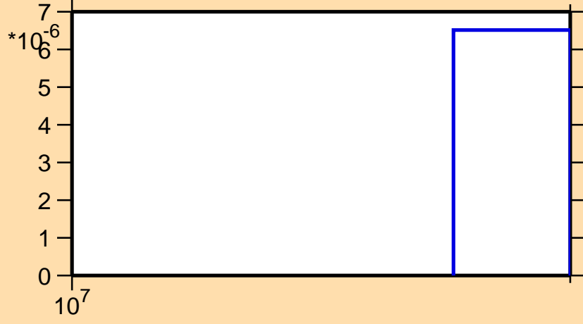
\sigma vs. E for ^{25}\text{Mg}(n,\text{nd})
