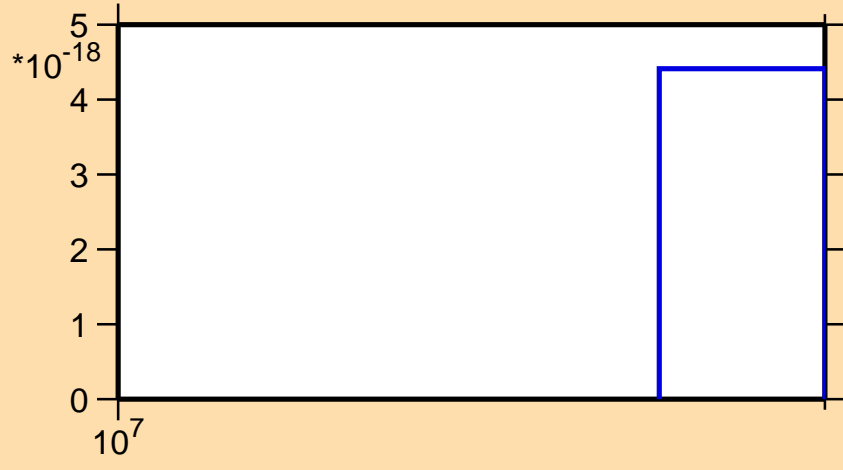
\sigma vs. E for ^{53}\text{V}(n,2n\alpha)
